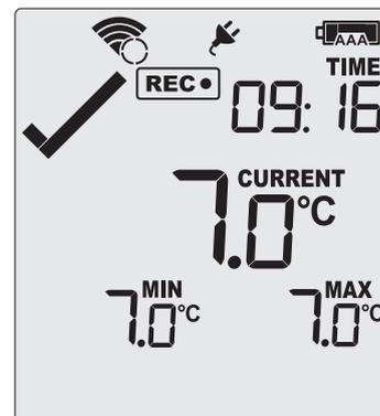
Once the UTRED30-WiFi has successfully connected to the wireless network (the WLAN symbol shows a tick) it will attempt to connect to the LogTag<sup>®</sup> Online cloud server (Cloud symbol shows an empty circle).
