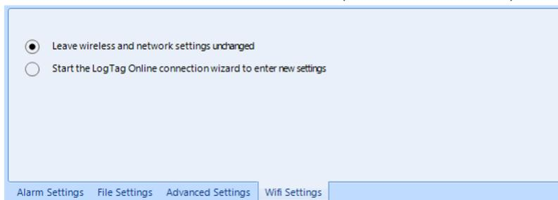
Select **Leave wireless and network settings unchanged** if you are only changing the logging parameters, but want the UTRED30-WiFi to connect to the same network as before. Selecting this option will retain the wireless and network parameters currently stored inside the unit.
