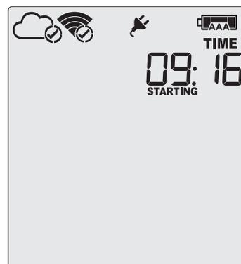
Once **READY** disappears, release the button within two seconds. **STARTING** will now disappear, and the **REC•** symbol will be shown. The UTRED30-WiFi now records temperature data.
