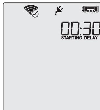
As with a regular push button start without delay, the UTRED30-WiFi will perform a [Connection Test](#) as soon as the recording has started. To check the connection before the delay value has elapsed, you can initiate the connection test yourself. Please refer to [Testing your wireless and network connection \(on page 19\)](#).
