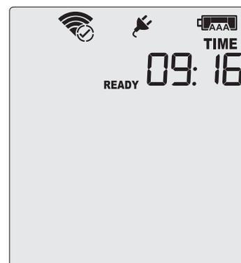
After successful completion of the wireless network test, the Wizard establishes a connection between the UTRED30-WiFi and the LogTag® Online cloud server. When completed successfully, the screen on the right shows.
