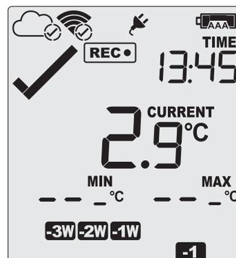
The logger will now track new min/max values. A min/max reset mark will be recorded in the logged data. As soon as the next reading is taken, both minimum and maximum values will be shown again.
