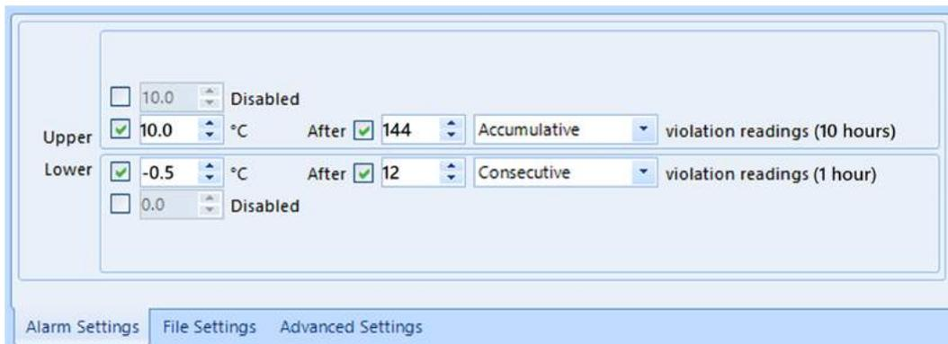
Once an alarm has triggered, the alarm indicator (x) remains shown until the alarm is cleared (see [Clearing an Alarm on page 33](#)) or the unit is reconfigured. The day alarm marker (T) remains shown until midnight, then it turns off and the marker for the previous day is shown (-1) to indicate the alarm was registered against what is now the previous day. When midnight passes next, this marker will move to and so on.
