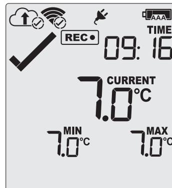
The logger has successfully completed its initial connection process. The Cloud and WLAN symbols remain to indicate that the last connection was successful.
