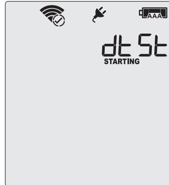
The UTRED30-WiFi will perform a [Connection Test](#) as soon as the recording has started. To check the connection before the start time is reached, you can initiate the connection test yourself. Please refer to [Testing your wireless and network connection \(on page 19\)](#).
