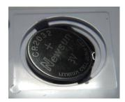
Press firmly down on the left hand side of the battery to click the battery into place.
