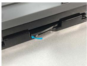
Plug the micro USB connector coming from the USB power supply into the interface's USB socket.
