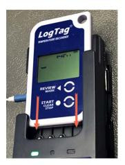
Any recorded data are now automatically transferred into the interface's internal memory. The green 'ready' LED will turn off and the red 'busy' LED will turn on during the data exchange.
