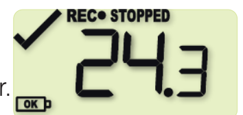
Figure 18: HAXO-16BT display with STOPPED visible while user is holding the START button
