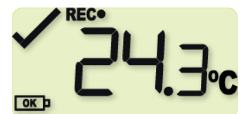
Figure 11: Logger has started recording
